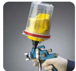
Connect air line to gun and purge air from the liner, adjust spray pattern and you're ready to spray.
