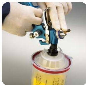
Mount the adapter flush to the lid tower base by pressing down firmly on the spray gun.
