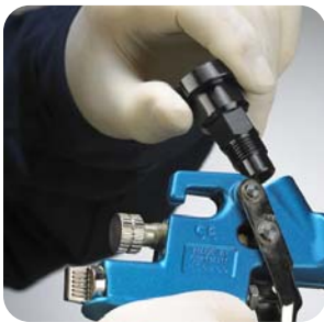
Thread the Carborundum adapter to the spray gun.
