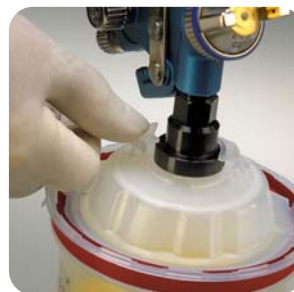
"Snap" the adapter locks over the adapter base to secure the lid to the gun adapter.
