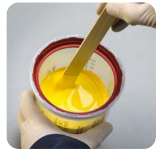
Mix paint by stirring (if not using a shaker) and clean liner flange/ring area of any paint before attaching to lid.
